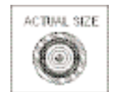
75 Ohm Coax: 16 AWG OFHC conductor with low-density unsintered PTFE tape, inner braided shield, PFA isolation layer and aluminum/mylar foil shield under a bare copper outer braided shield and then jacketed with PVC to 0.383" O.D.
