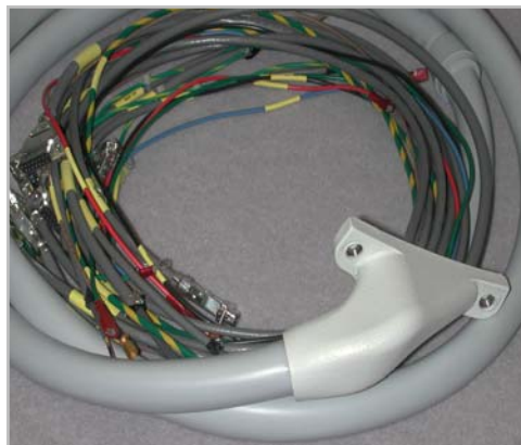
HV cable/control harness for C-Arm equipment.
