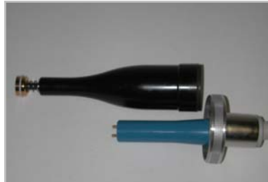
ML style bi-plug shown with "coke bottle" adapter used in Seifert and Philips tube towers. PMI integral "coke bottle" termination eliminates bi-plug/adapter combination which frequently results in premature burnout of contacts due to electrical instability and overheating.
