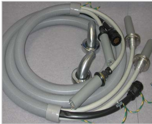
C-Arm harness in flexible "old-style" hose with federal standard terminations.
