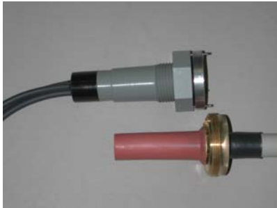
H435 mini plug with recessed pins molded from EPR for vulcanized termination to cable insulation. Rated for 75kV, 1-4 conductors. Shown with H1541 P2 cathode receptacle.
