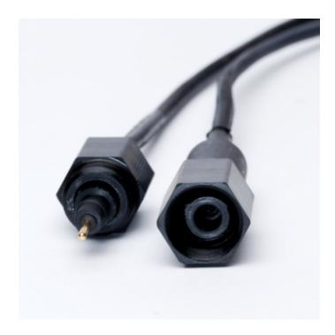
BIRNS Rubber Connectors are simple, low-cost cable connectors for light-to-medium power or signal applications, and/or for applications where weight and/or magnetic signature are considerations. They are rated to 1,000m and 500VDC, and made of a durable elastomer that cannot chip or dent. They mate with each other in the in-line mode, and with BIRNS Polymeric Series bulkhead connectors. They are well engineered, yet extremely affordable and easy to use.
